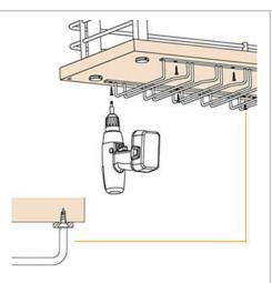
**Important:** Length (L) measurement is hole centre to hole centre, allow additional 30mm for installation.
